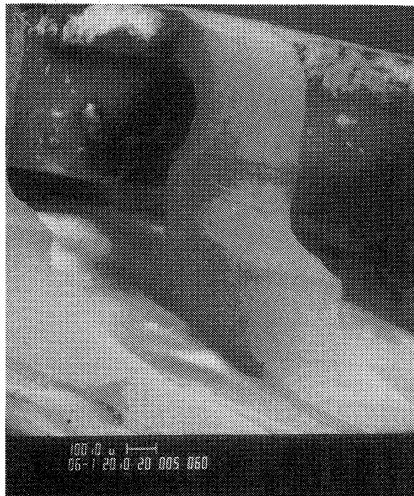
Solder Joints on a SO-14 Package on PCB
